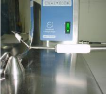
Pic 7. probe placed in the housing at the base of the pot
